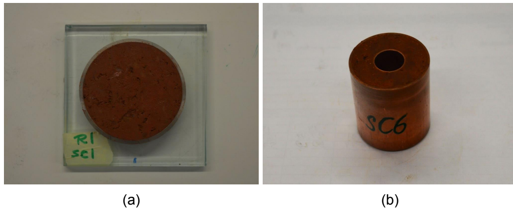
Figure 6.9: (A) Compacted shrinkage test sample of AS soil after retrieving from compaction mould and preparation and (B) CT cell with cored soil sample after retrieving from the compaction mould and preparing for dielectric measurement.
