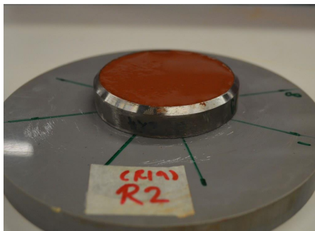
Figure 6.13: Photograph of the AS sample in the early stage of the shrinkage test.
