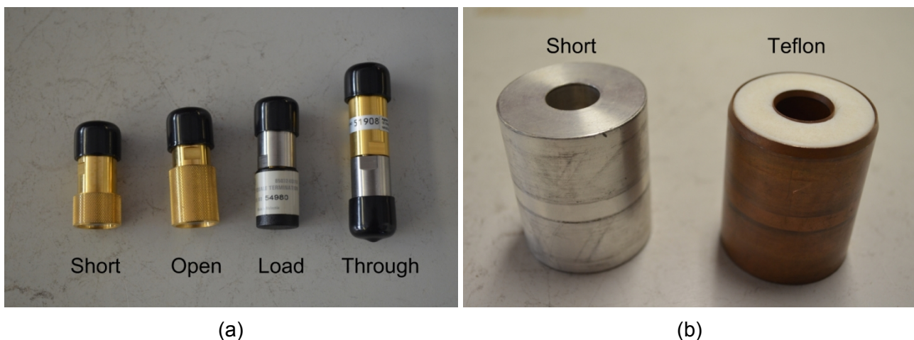
Figure 6.5: (A) Mechanical calibration kit (Agilent type N 85032F) that includes open, short, load and through calibration standards and (B) additional two standard calibration materials – Teflon and short – used to check the performance and success of the VNA calibration.
