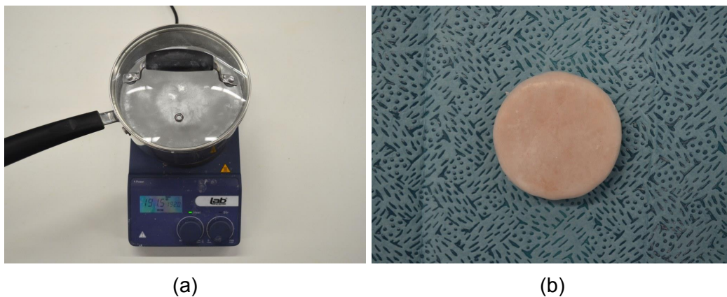
Figure 3.2: Preparation steps for water displacement method according to ASTM D4943-08 [1], ASTM D7263-09 [2]: (A) melting process of a paraffin block in a pot on a hot plate, (B) prepared soil sample with a wax coating
