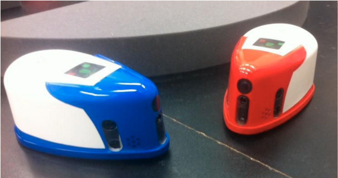
Figure 4.1: This photo shows two iRat robots meeting to play a language game. The iRats have differential drive (not shown) and a forward facing camera that looks through the top of the 'i'.
