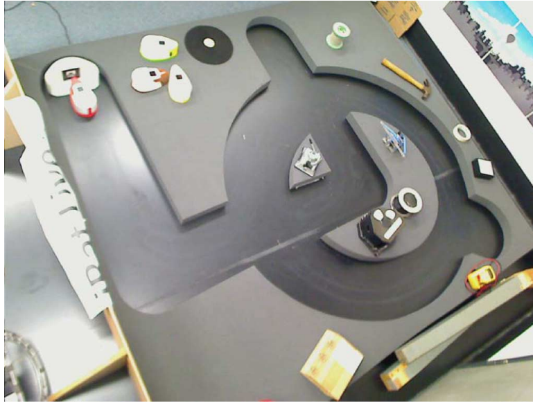
Figure 5.5: The environment used for the iRats language studies. It is created from a U and a Q cut from a foam sheet.
