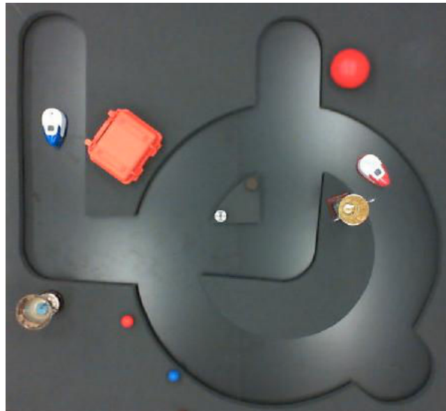
Figure 4.2: The maze used in the study as shown from the overhead camera used to establish shared attention between the robots. The blue iRat is in the left side of the U and the red iRat is in the right side of the Q. Visual features have been placed around the edges of the maze to enable the mapping system to create coherent maps of the maze.
