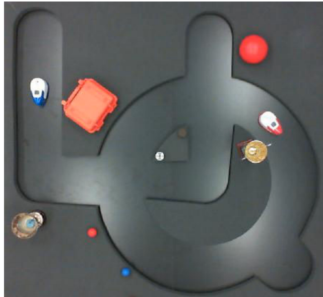
Figure 3.5: The UQ maze environment. The UQ maze consists of an interlocking “U” and “Q” to create loops that are a suitable for correction using SLAM. Visually distinct objects are added to the UQ maze to assist SLAM.
