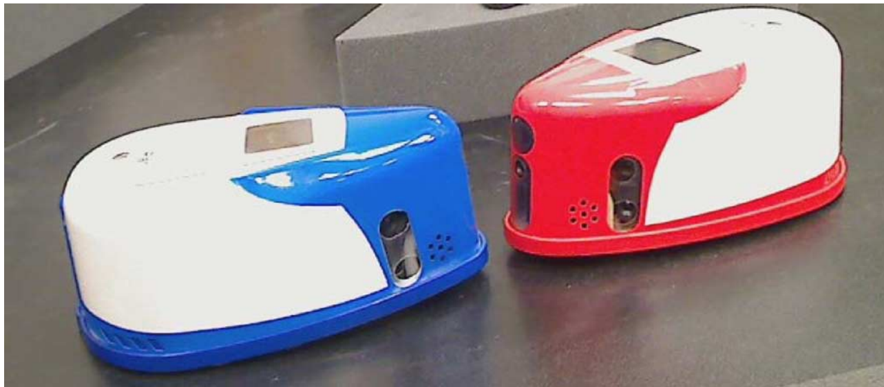
Figure 5.4: iRats talking. iRats randomly explore their environment until they meet. When they are within hearing distance of each other, they stop, and have a conversation.
