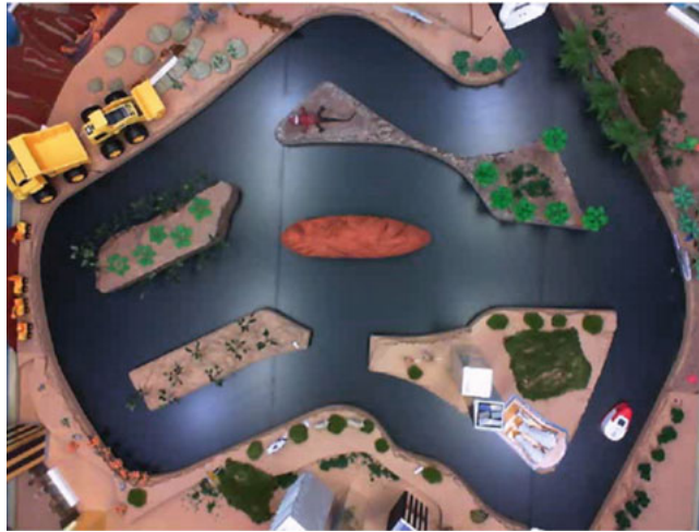
Figure 3.6: The Australia maze environment (reproduced from Ball et al. (2013)). The Australia maze was designed by UQ’s School of Journalism and Communication for iRat SLAM studies. The Australia maze measures 2.5 \times 1.8\text{m}
