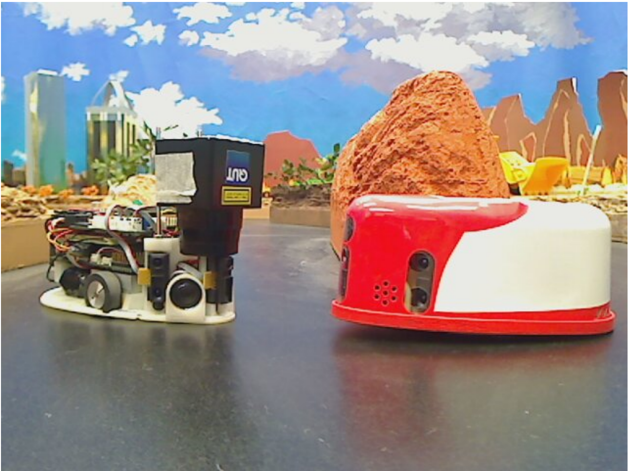
Figure 6.1: Lingodroid iRats in conversation. On the right is a standard ‘camera iRat’ which has a forward facing camera inside the dot of the ‘i’. On the left is the modified ‘laser iRat’ which has a laser scanner mounted upside down. The standard iRat’s cover has been removed to fit the laser scanner. The two iRats are shown in the environment used for the studies in the chapter (also see Figure 6.2).
