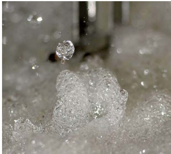
(b) Details of air-water structures and droplets at the roller surface (high-shutter-speed photograph) Figure 1 – Air entrainment and macro-scale bubble-turbulence interaction in strong hydraulic jump with partially-developed inflow conditions (see Test 2 in Table 1 for flow conditions)
