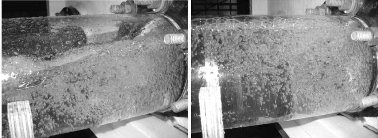
Figure 5 – Flow patterns in Exit Pipes. Left shows high flow rate, high tail-water. Right shows low flow rate, low tail-water.
