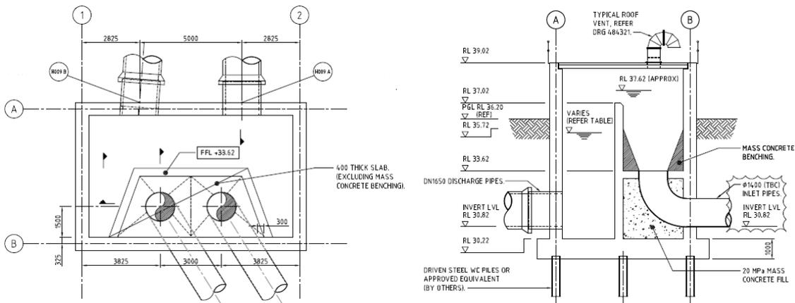
Figure 1 – Original Design of Weir Chamber
