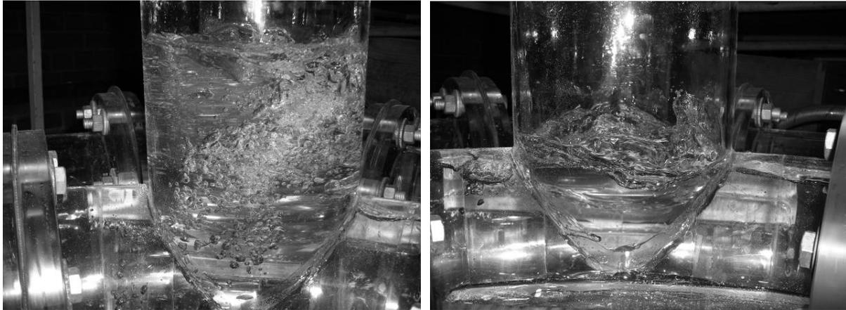
Figure 6 – Flow in the Air Releases. Left shows high flow rate, high tail-water. Right shows low flow rate, low tail-water.
