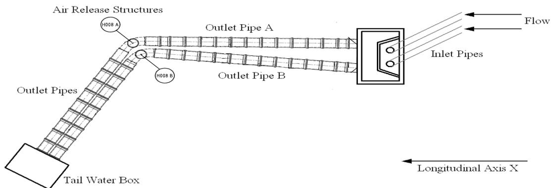
Figure 2 – Layout of the Components Investigated showing Chamber, Pipelines and Air Release Structures.
