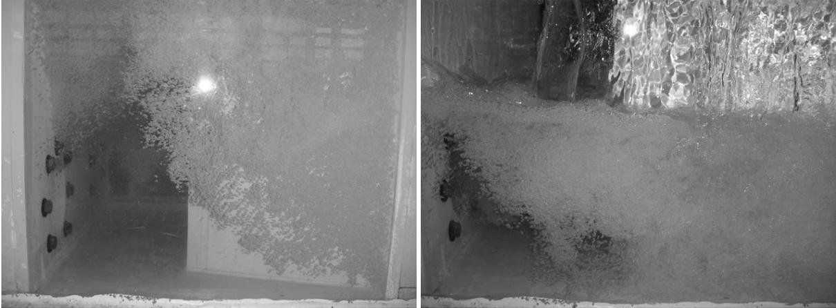
Figure 4 – Flow patterns in the Chamber. Left shows high flow rate, high tail-water. Right shows low flow rate, low tail-water.
