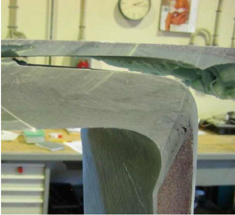
Figure 4 Delamination - faulty injection
