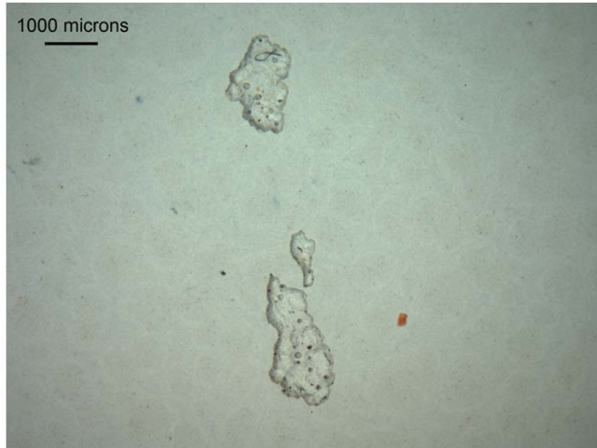
Figure 3.6 Optical microscopy of water jet erosion failure of Coating A applied on flat steel panels and using a water nozzle-coating distance of only 5 cm (Experiment 4).
