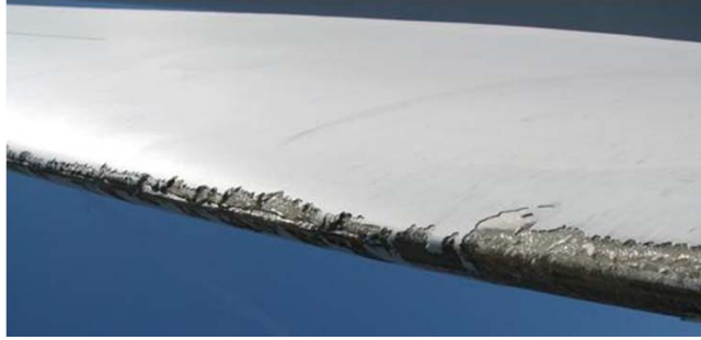
Figure 1.7 Leading edge erosion of a wind turbine blade. Reproduced from [21].
