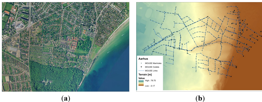
Figure 7. Study area located in Aarhus, Denmark. The area is a fully developed residential area with a combined sewer system. (a) shows an orthophoto while (b) shows the digital surface terrain as well as the sewer layout.
