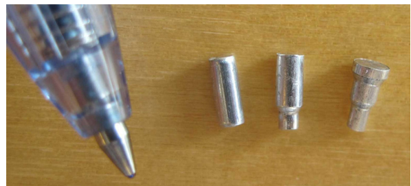
Fig. 5. Specimen at different forming stages.
