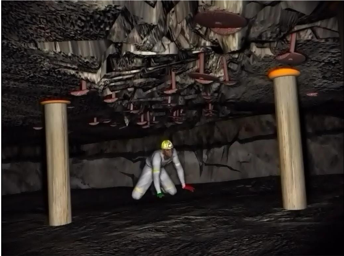
Figure 7.19: A miner in the unsupported area of blocky ground in the stope face area.
