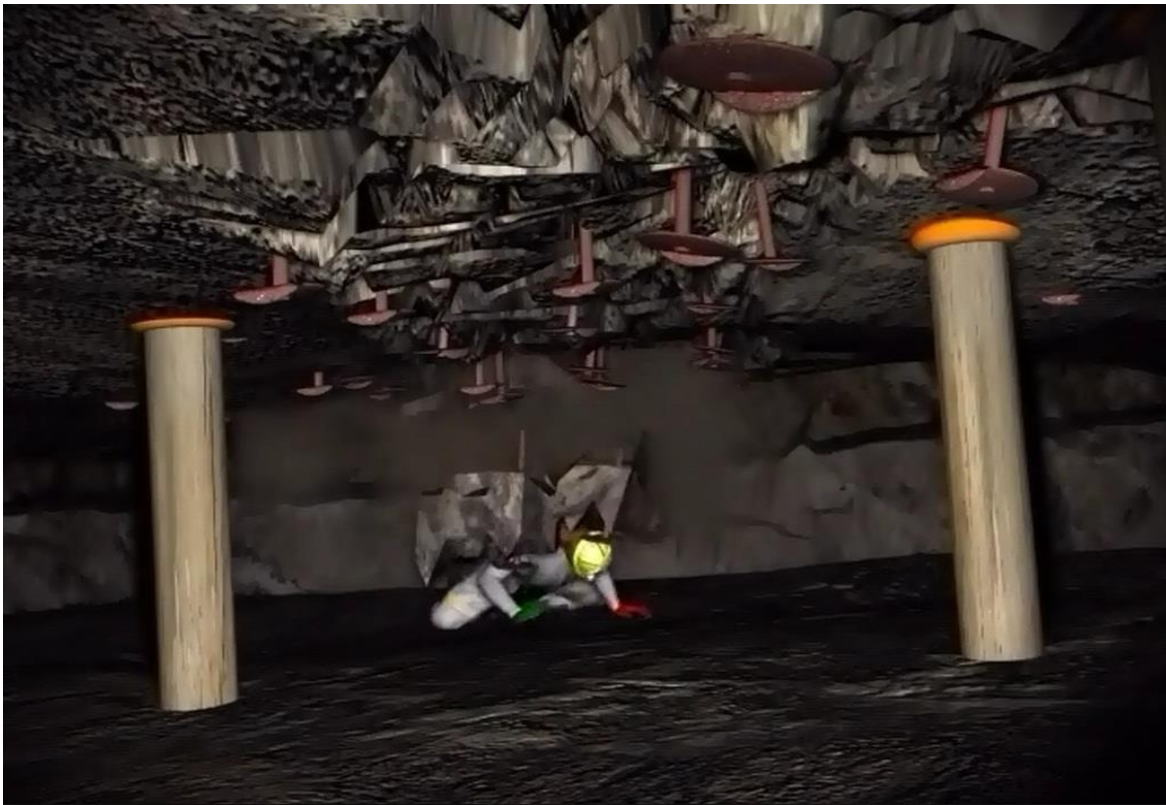
Figure 7.20: A fall of ground occurs, injuring the miner.
