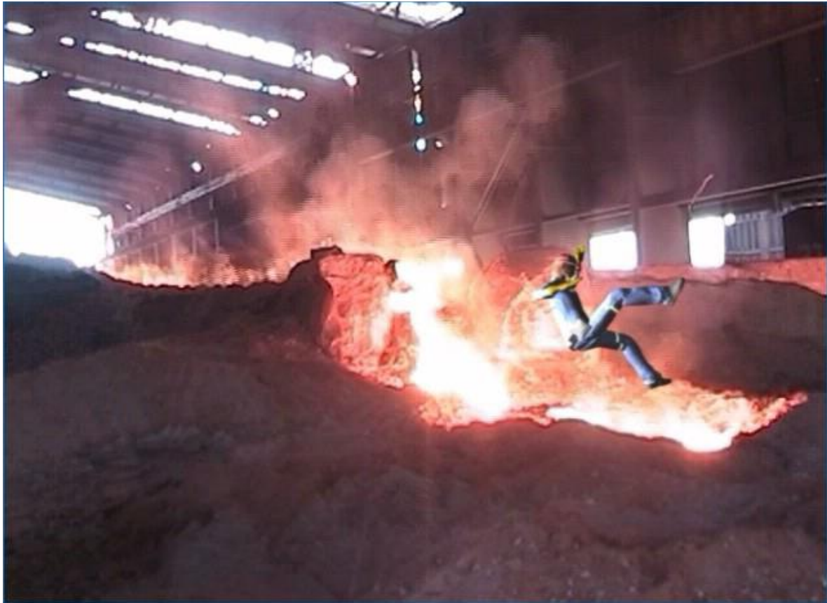
Figure 2.10: Worker attempting to jump over hot slag (Van Wyk & De Villiers, 2009).
