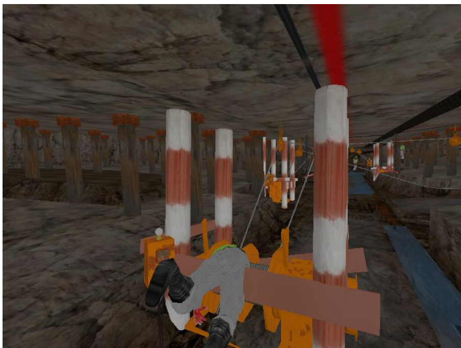
Figure 6.18: Miner being pulled into the winch as a possible consequence of operating the winch without drum guards.
