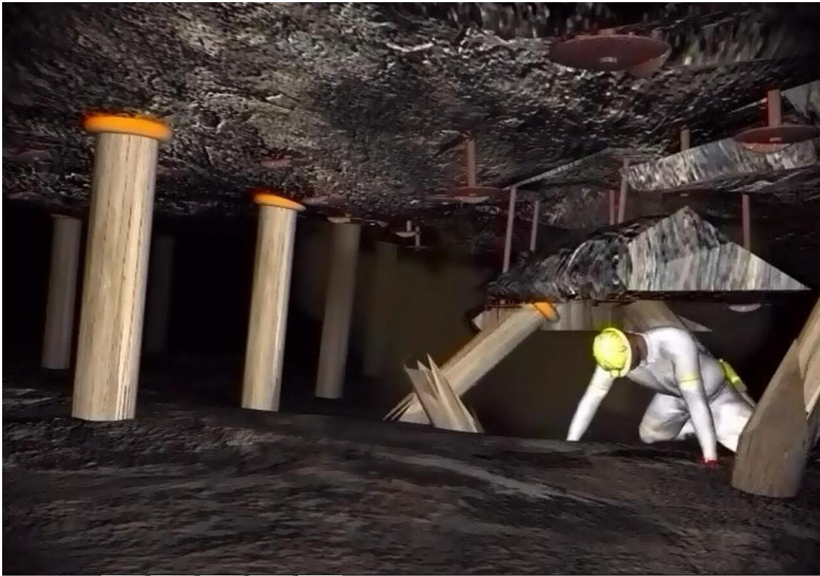
Figure 7.21: A fall of ground in an incorrectly supported area.
