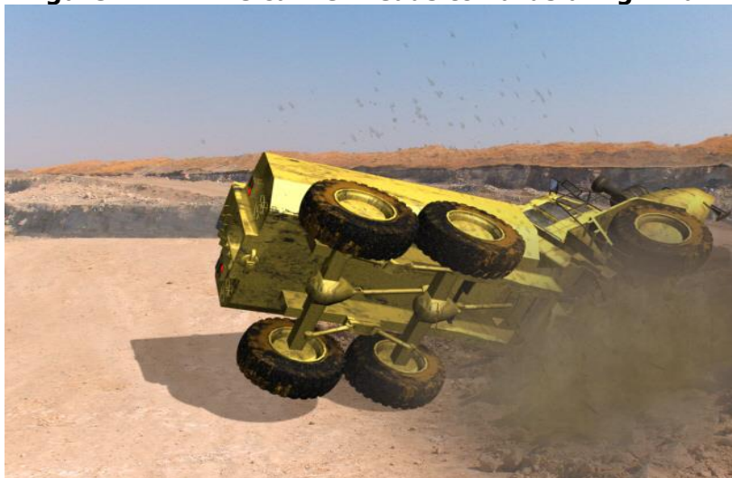
Figure 2.7C: The water carrier hits a sidewall and starts to overturn.
