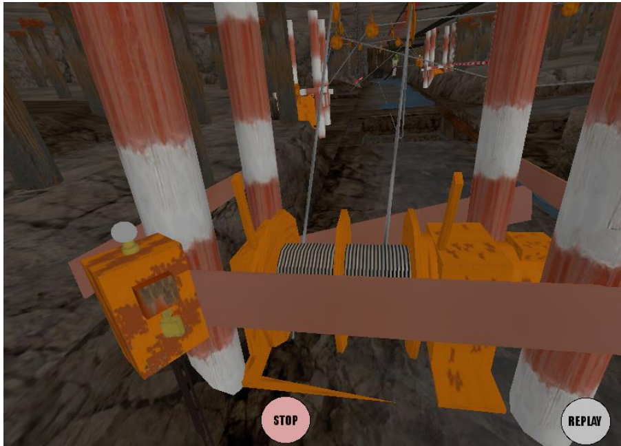
Figure 6.17: No drum guards on the winch.
