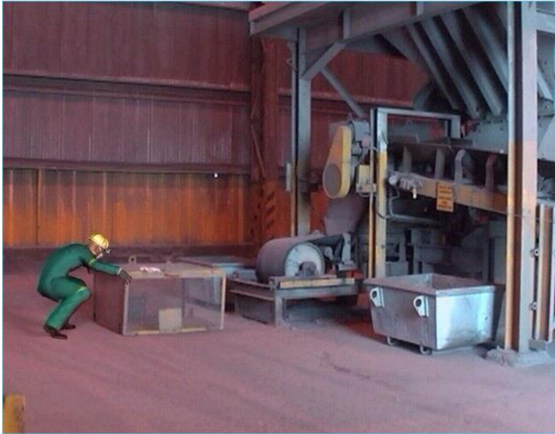
Figure 2.9: Worker removing the drum guard while conveyor is running (Van Wyk & De Villiers, 2009).
