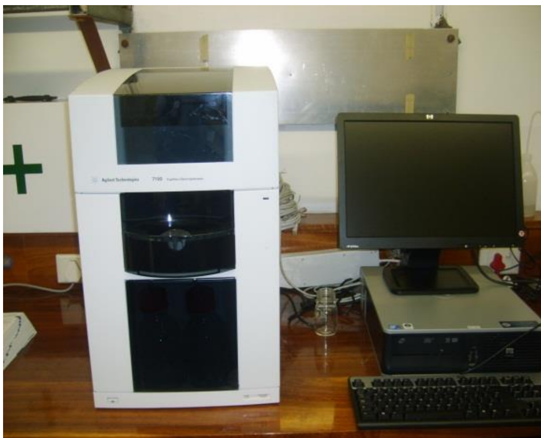
Figure 4.7. Agilent 7100 Capillary electrophoresis system used in the study
