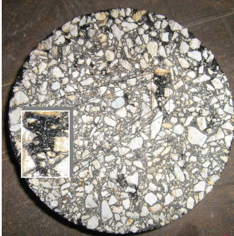
Figure 32. Surface Voids Present on External Trimmed IDT Specimens
