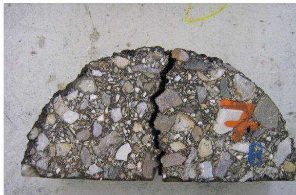
Figure 74. RSCB: 10Hz, 30% Load Typical Specimen Failure
