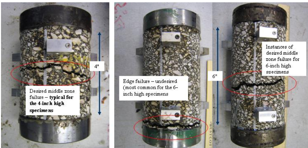
Figure 20. Example of DT Failure Modes
