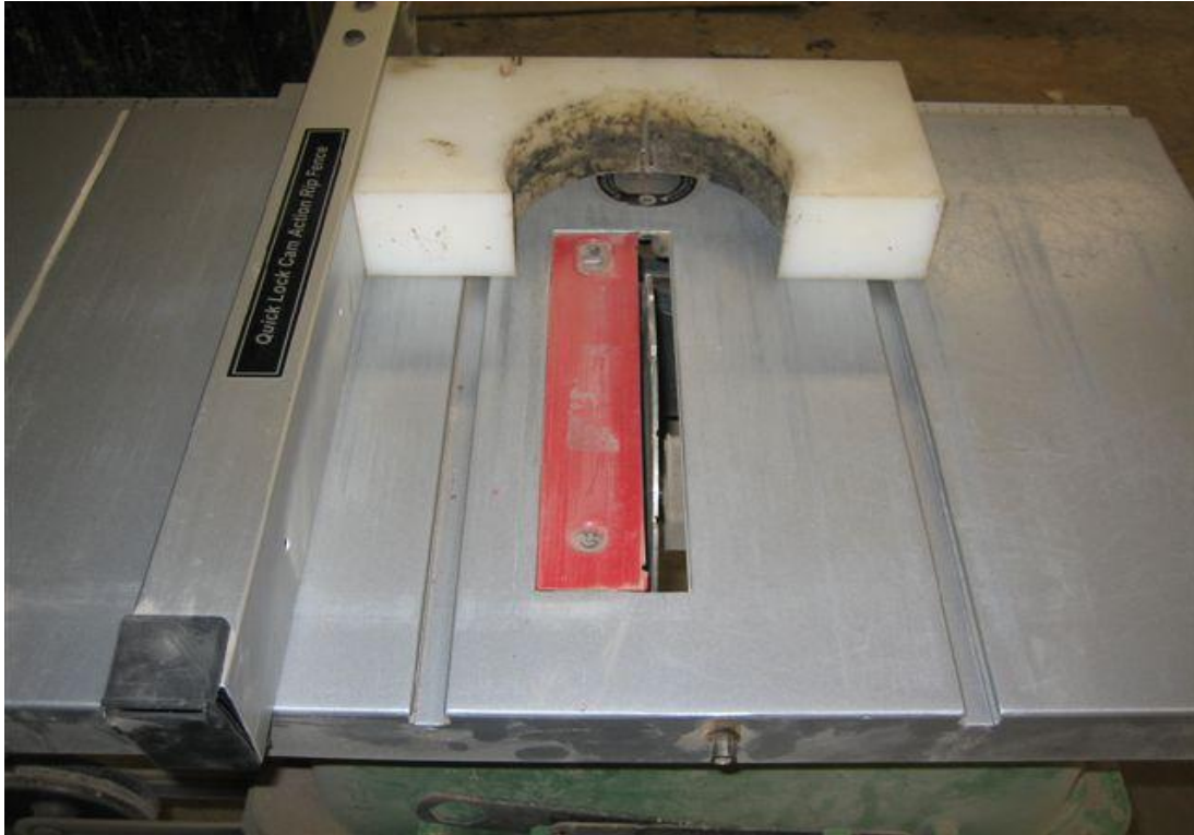
Figure 33. Equipment Used to Notch SCB Specimens
