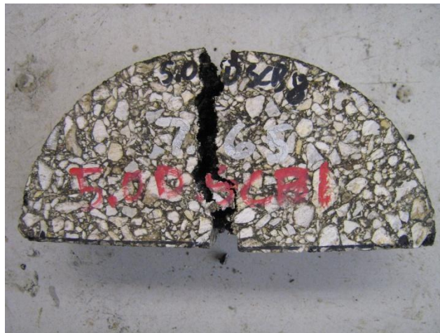
Figure 75. RSCB: 1Hz, 25% Load Typical Specimen Failure
