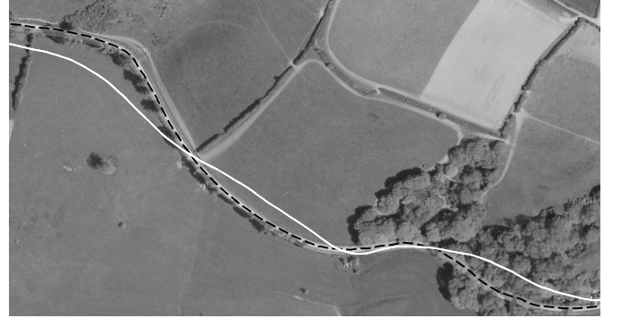
Figure 3: The estimated vehicle track (in white) plotted over a map of the road travelled, with the true path shown as a black dashed line, as calculated from the FoE motion shown in figure 2.
