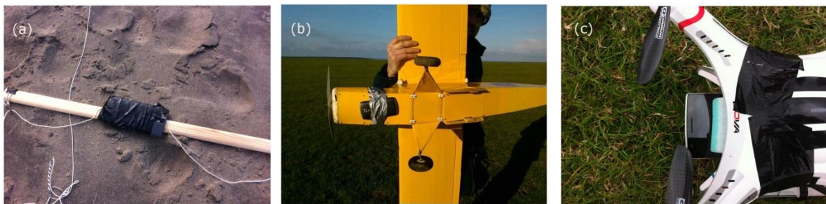
Figure 2: examples of basic fitting methods to hold the mobile phone handset in place on airborne platforms. Shown are (a) a wooden bar suspended from two strings on the flexifoil stunt kite with the OnePlus One phone attached using hardware tape (b) the Acer Liquid Z3 taped to the underside of the balsawood Flair Cub aircraft with hardware tape and (c) the OnePlus One phone attached using hardware tape to the underside of the Quantom Nova lightweight quadcopter with a sponge to reduce image blurring caused by airframe vibration.
