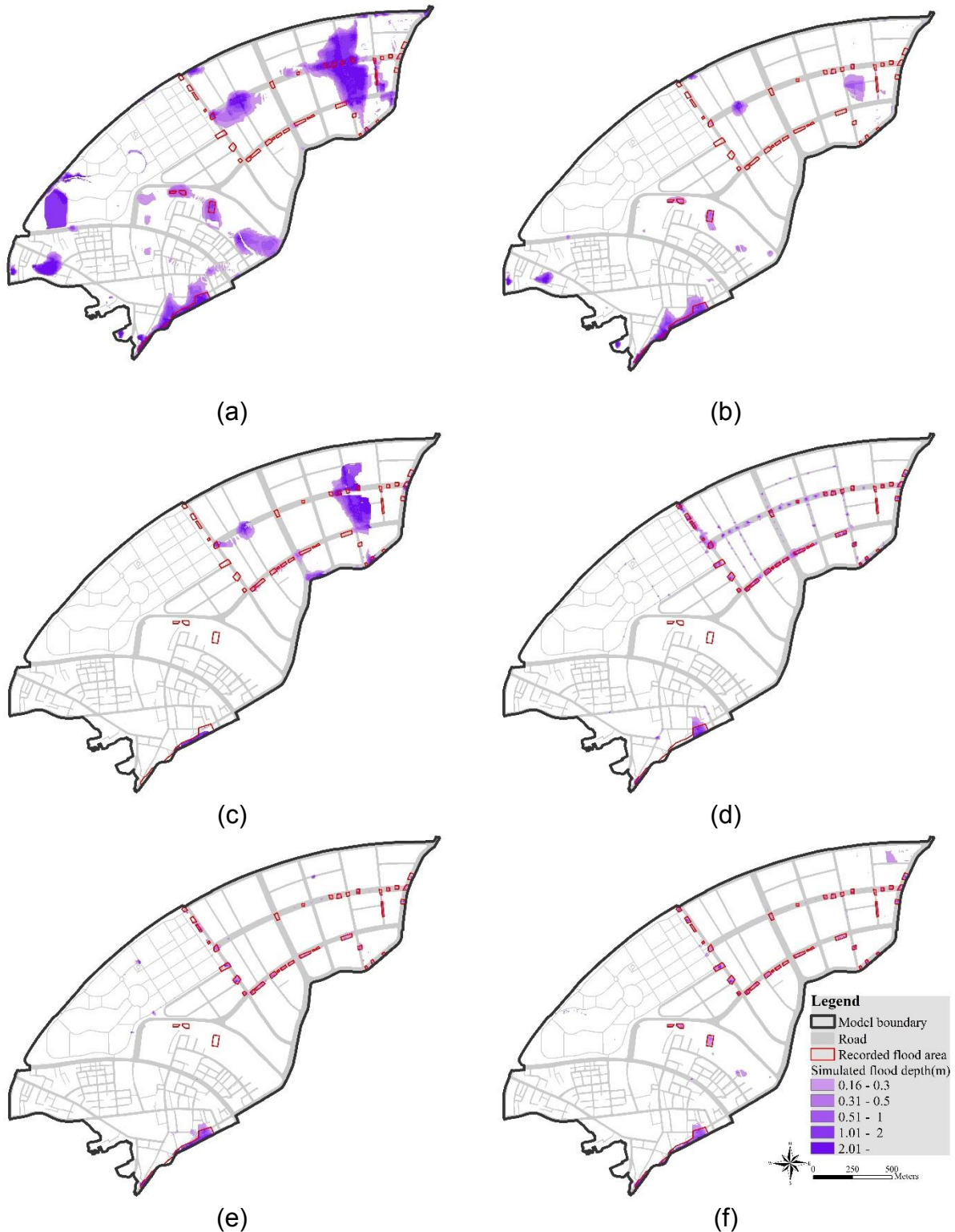
Figure 11 shows the modelled flood extents of the six approaches and the recorded flood areas (red boundary polygons) of a simulated event. Although the ACCs of the 2D OFM only approach for all the simulated events were around 0.85, the results of other approaches were obviously better (above 0.94). The 2D OFM only approach
