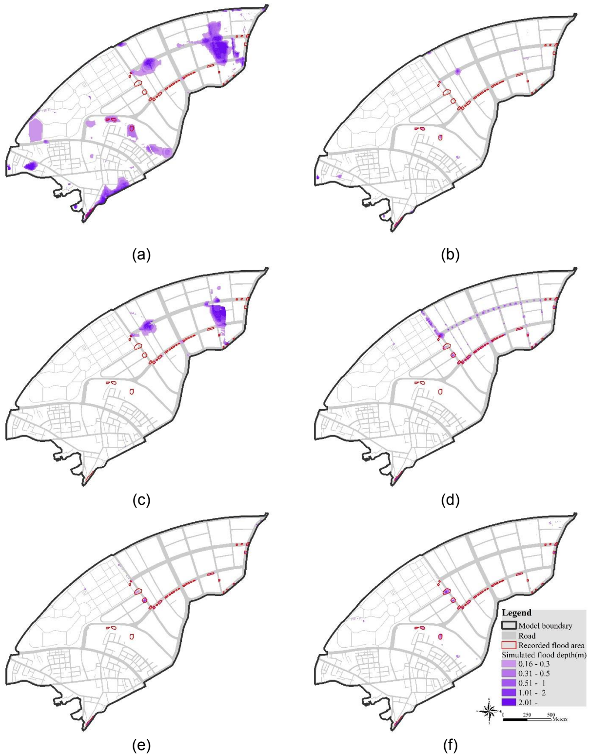
Figure 10 The modelled flood extents of the six approaches and the recorded flood areas (red boundary polygons) for Typhoon Meari (2011), (a) the 2D OFM only, (b) the 2D OFM with rainfall reduction, (c) the combined SFM/OFM, (d) the coupled SFM/OFM, (e) the coupled OFM/SFM, and (f) the mixed SFM/OFM and OFM/SFM coupling.
