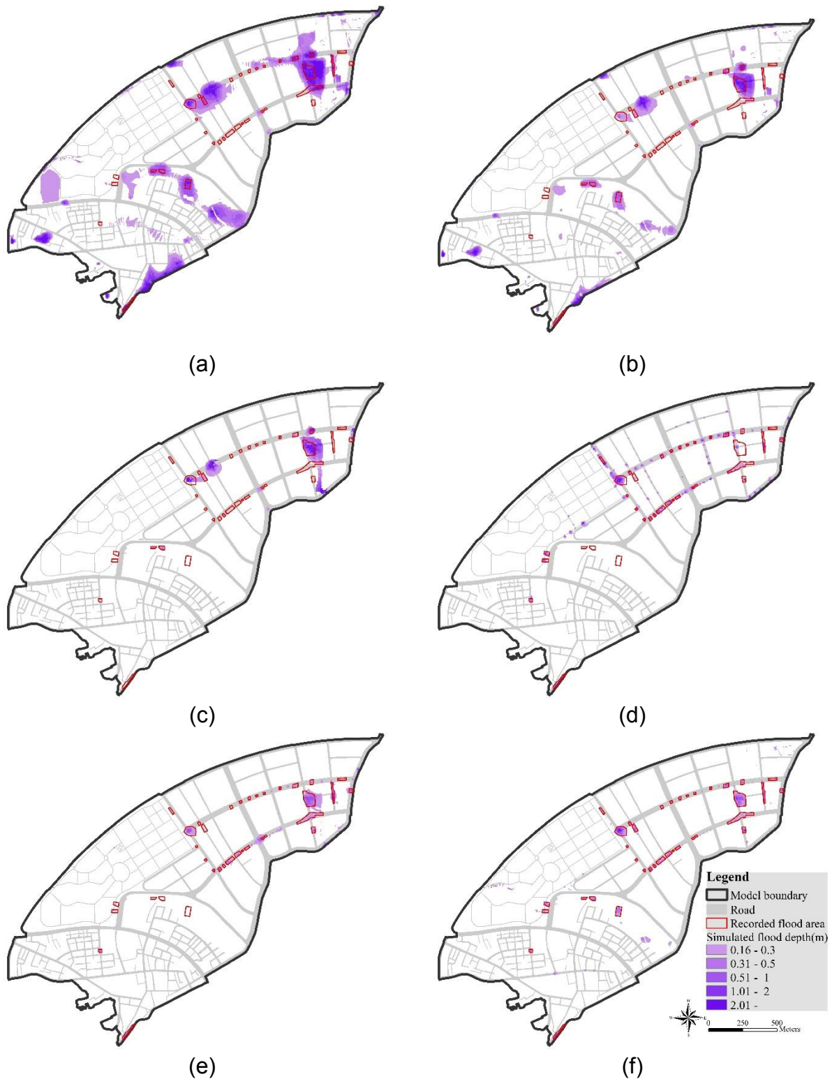
Figure 9 The modelled flood extents of the six approaches and the recorded flood areas (red boundary polygons) for the 15 June 2012 event, (a) the 2D OFM only, (b) the 2D OFM with rainfall reduction, (c) the combined SFM/OFM, (d) the coupled SFM/OFM, (e) the coupled OFM/SFM, and (f) the mixed SFM/OFM and OFM/SFM coupling.
