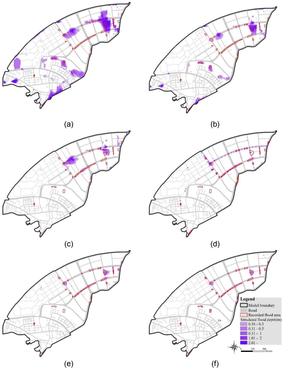
Figure 8 The modelled flood extents of the six approaches and the recorded flood areas (red boundary polygons) for the 12 June 2012 event, (a) the 2D OFM only, (b) the 2D OFM with rainfall reduction, (c) the combined SFM/OFM approach, (d) the coupled SFM/OFM approach, (e) the coupled OFM/SFM approach, and (f) the mixed SFM/OFM and OFM/SFM approach.
