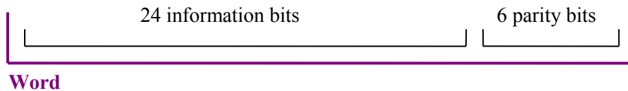
Figure 3: GPS L1 C/A navigation message word structure
