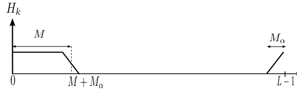
Figure 4.16: Spectral shaping filter with root raised cosine
