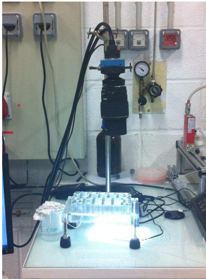
Figure 1.1: Experimental apparatus - the microchannel is horizontal and the image sequences are taken with a digital camera placed above.
