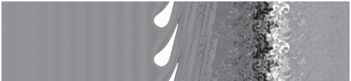
Figure 9.6 - Instantaneous field of the entropy wave at different times for the case where entropy is pulsed at the inlet. (a) t/\tau_0 = 0.1 , (b) t/\tau_0 = 0.2 , (c) t/\tau_0 = 0.3 .
