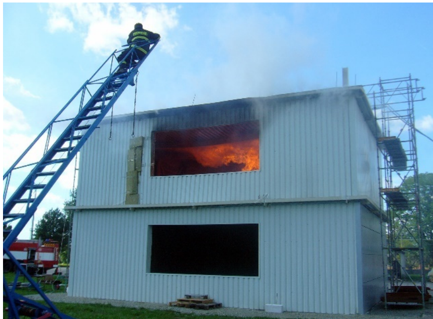
Figure 2.4. Experimental building during Veselí travelling fire test (photo provided by Horová K., CVUT in Prague).
