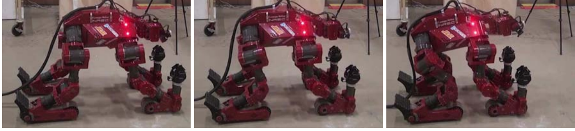
(a) CHIMP moving the frontal tracks backwards
