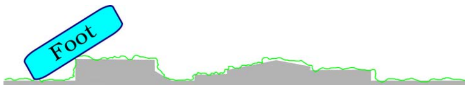
Figure 4.32 – Example of a situation handled by the approach. The gray part represents the real environment, and the green line the stereoscopic reconstruction. The foot is in its final position after the adaptation by the proposed method.
