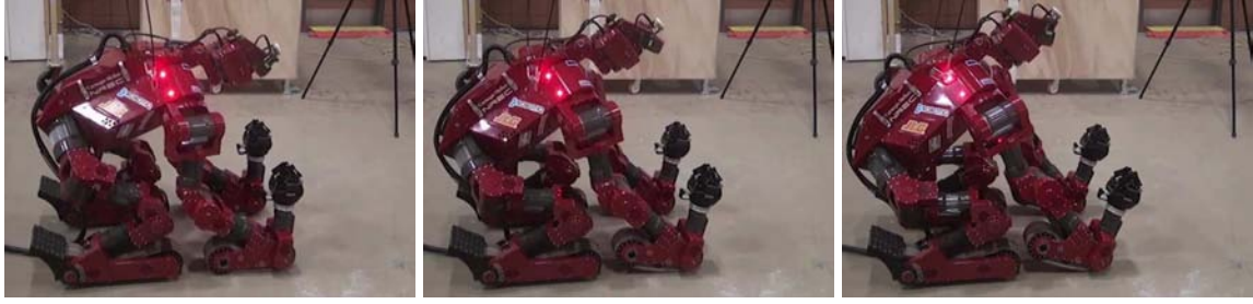
(b) CHIMP rotating the frontal tracks
