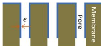
Figure 3.9: Schematic representation of pore size reduction after the photografting: polyRTIL layer in blue and support membrane in gray, e representing the graft layer thickness.
