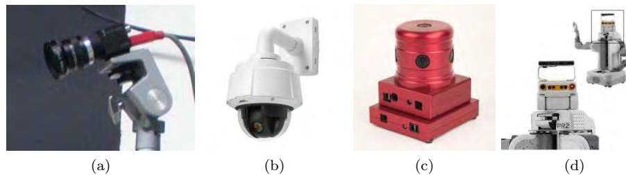
Figure 1.5: Examples of some perception sensors/systems. (a) A fixed view wall mounted classical camera; (b) a PTZ camera; (c) a Ladybug2 camera system that can capture spherical images, and (d) multiple cameras and a movable laser scanner mounted on the mobile robot PR2.
