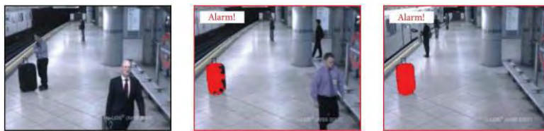
Figure 1.2: Automatic abandoned luggage detection [Porikli 2008].
