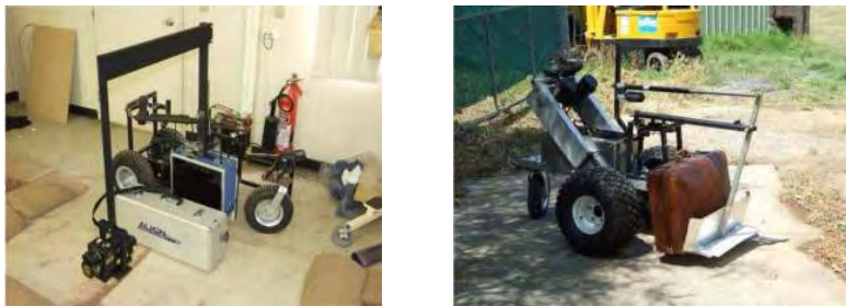
(a) An X-ray inspection robot.
