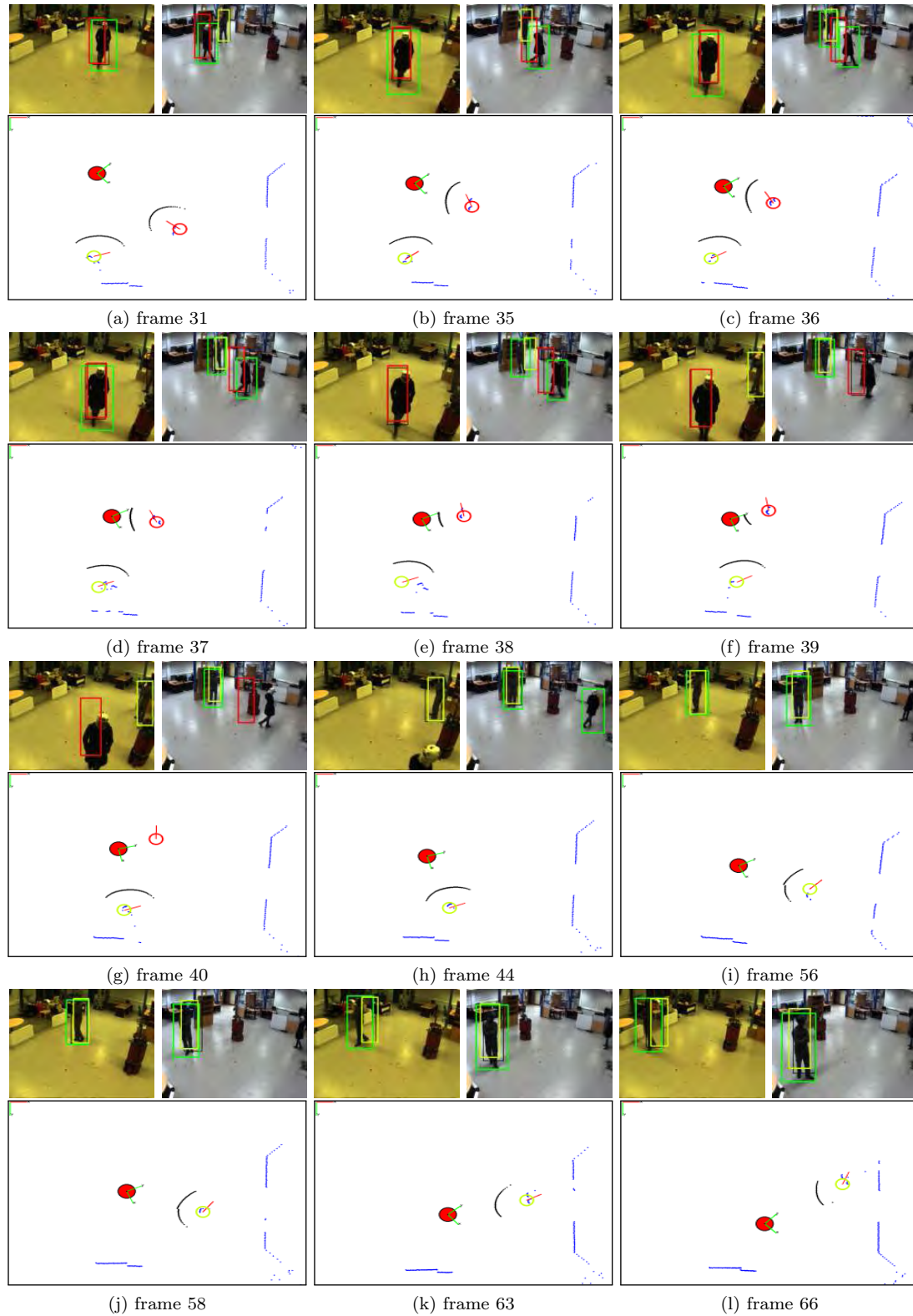
Figure 6.16: Sample robotic run for safe navigation evaluation with perception based on the GPU-HOG-BIPBoost detector. (Please see text for explanation).
