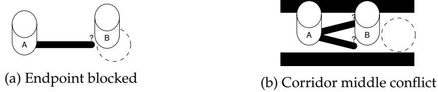
Figure 3.6: Cases where static planning fails due to agent B blocking collision free solutions for Agent A to goal.
