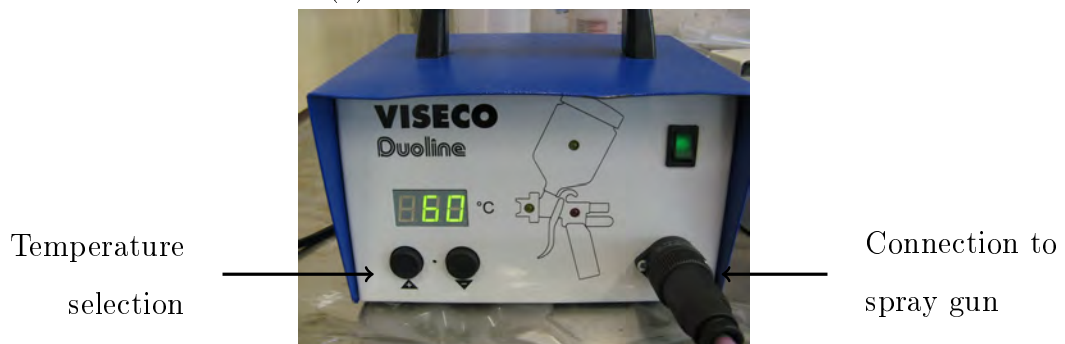
(c) Gun temperature control unit
