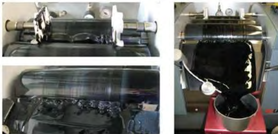
Figure 3.1 – Three-Roll Mill during calendering procedure
