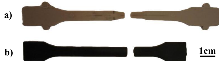
Figure 3.14. Test beams after the tensile measurements a) PEEK b) PEEK with 1wt% of CNTs.
