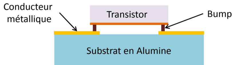
Figure IV.2: Vue transversale d'un report flip-chip.
