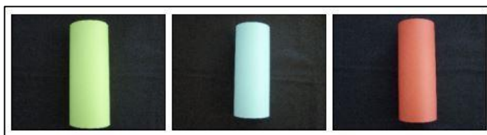
Figure 2.7: Landmark colours made out of A4 cardboard coloured paper; have 40 mm in radius and 210 mm in height [4].
