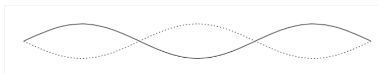
Figure 2.6: The string is divided into three equal length section.
