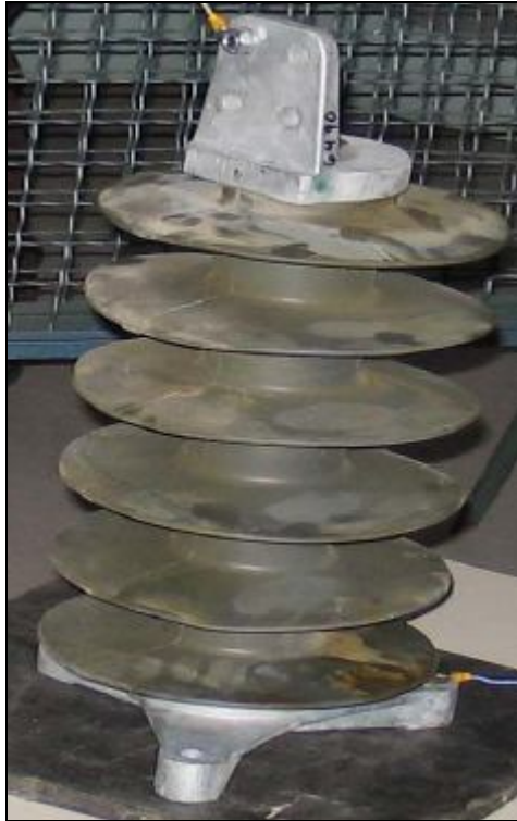
Figure 2.1: A ZnO surge arrester
