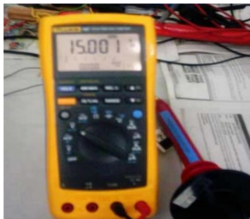
Figure 2.13: Output Voltage of the DC Power Supply [22]
