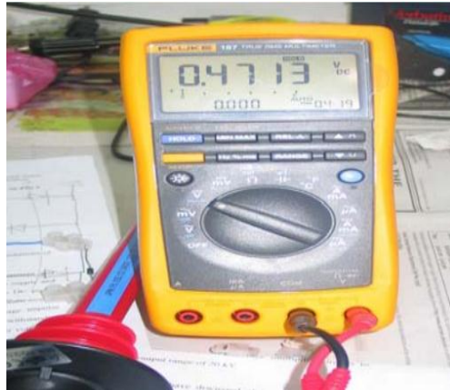
Figure 2.12: Experimental Output Voltage of Doubler Circuit [22]
