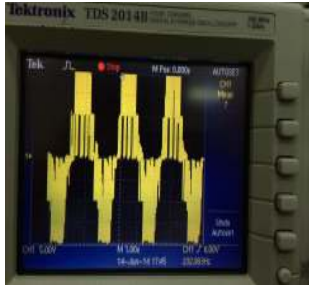
Figure 17: Phase voltage at no load
