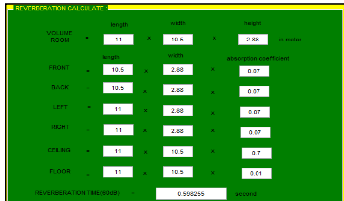
Figure 6. Results of the GUI system developed to calculate reverberation time
