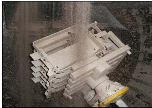
Figure 2.1: Stuccoing process of ceramic shell mould by rainfall sand technique [13]
