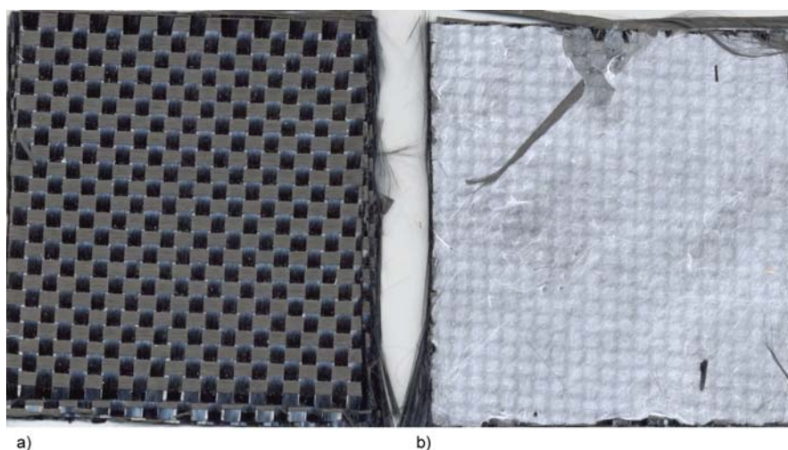
Figure 2. Carbon plain weave fabric without (a) and with (b) PAN nanofiber veil
