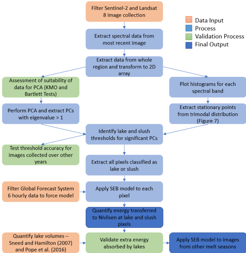
Figure 4. Flow chart of overall method applied in this study for quantification of energy contribution of SGL and slush areas on Nivlisen Ice Shelf.
