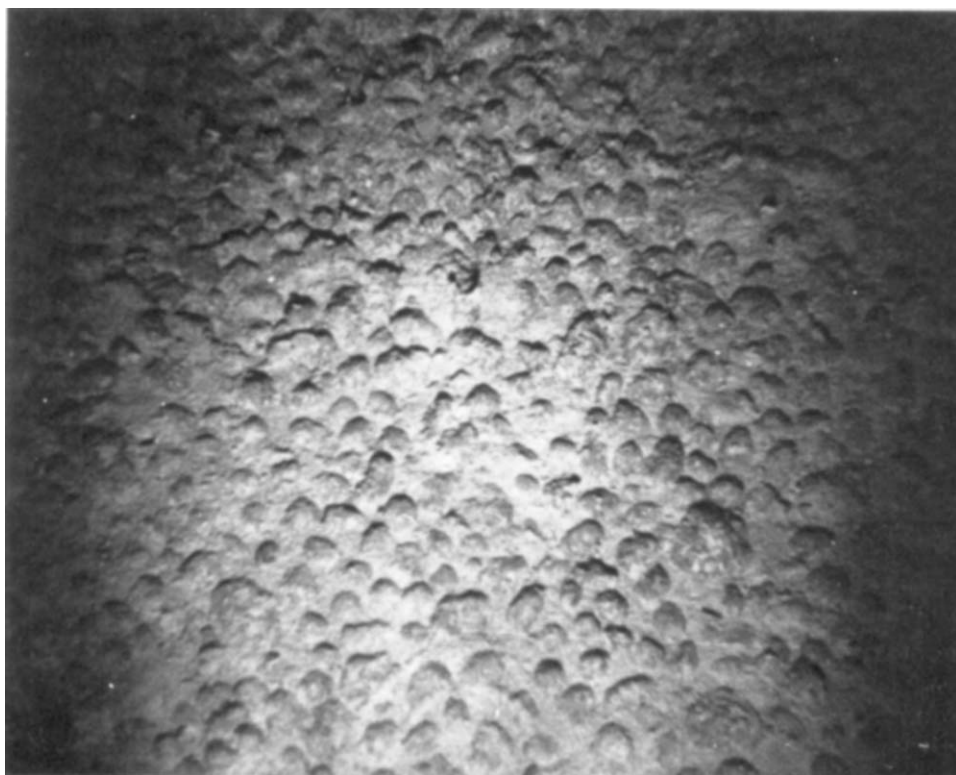
Fig. 11-1. A sea-floor photograph taken in 3,778 m of water at 20^\circ 00' \text{N } 113^\circ 57' \text{W} . The photograph covers a sea-floor area about 160 cm by 160 cm. The nodules average about 6 cm in diameter and the coverage would be about 80%. The concentration estimate is 30 \text{ kgm}^2 . (Photograph by N. Zenkevitch, Institute of Oceanology, Moscow, U.S.S.R.)
