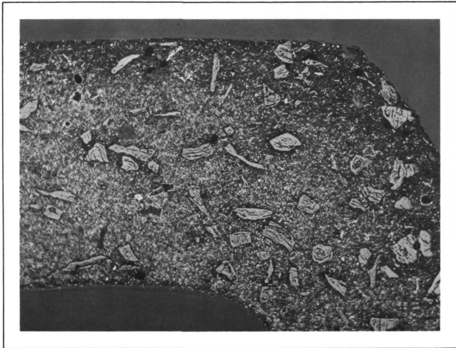
Unsintered Tungsten-Uranium Dioxide Tube (150X)
