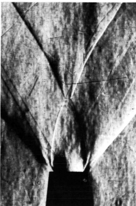
(a) Ratio of base diameter to maximum diameter, 0.385; nozzle-pressure ratio, 16.0.
