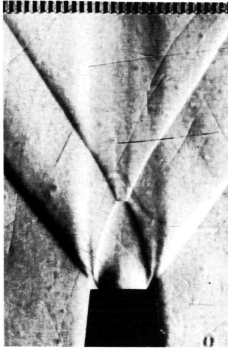
(b) Ratio of base diameter to maximum diameter, 0.385; nozzle-pressure ratio, 10.0.
