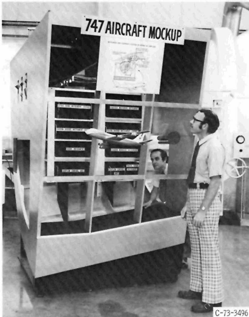
Figure 2. - Full scale mockup of area selected in 747 for GASP measuring equipment.
