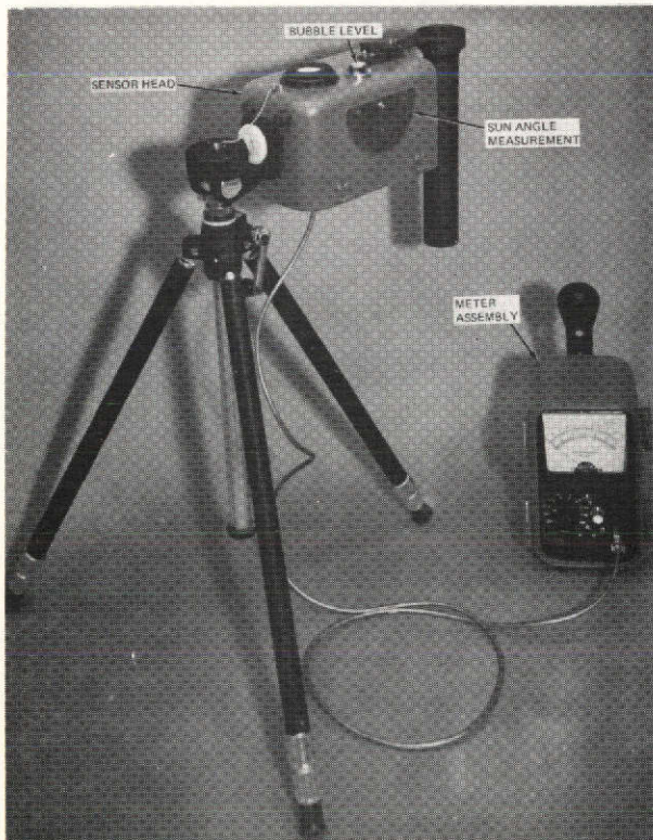
Global Irradiance ( H ) — 2\pi steradian field of view for measuring downwelling (incident) radiation ERTS MSS bands. Bubble level aids this measurement.
