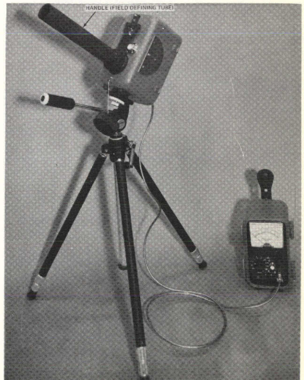
Reflected Radiation — Used with small calibration panels and cards, to obtain direct measurement of truth site reflectance. Reflectance also immediately derived from ratio of reflected radiance and global irradiance.
