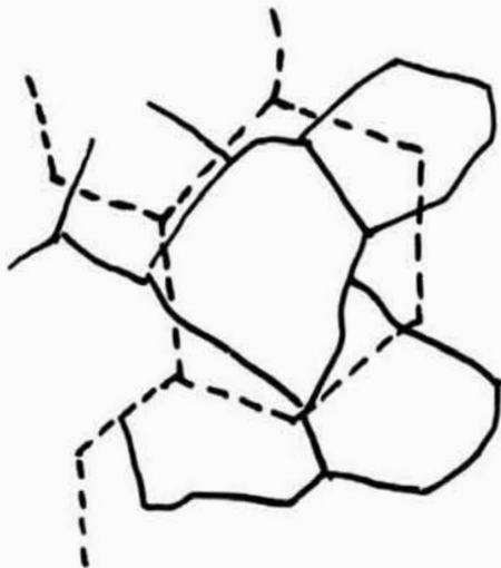
Fig. 22 Equiaxed Surface Grains and Interior Grain Structure (Surface Morphologies)
