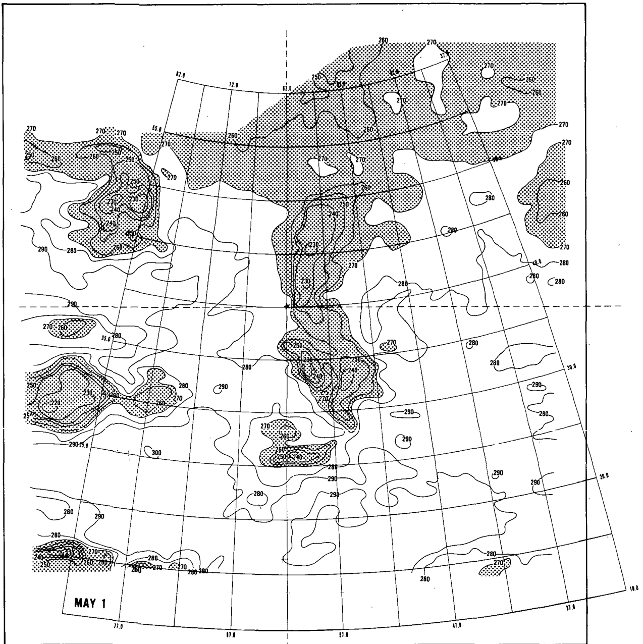
Figure 3.—Radiation maps for May 1, 1969. (a) 10- to 11- \mu\text{m} . Isotherms are in ^{\circ}\text{Kelvin} .
