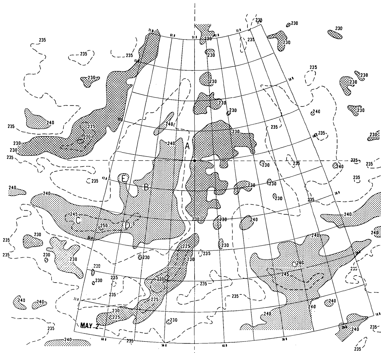
Figure 6 (continued).—Radiation maps for May 2, 1969. (c) 6.5- to 7.0- \mu\text{m} . Isotherms are in ^{\circ}\text{Kelvin} .
