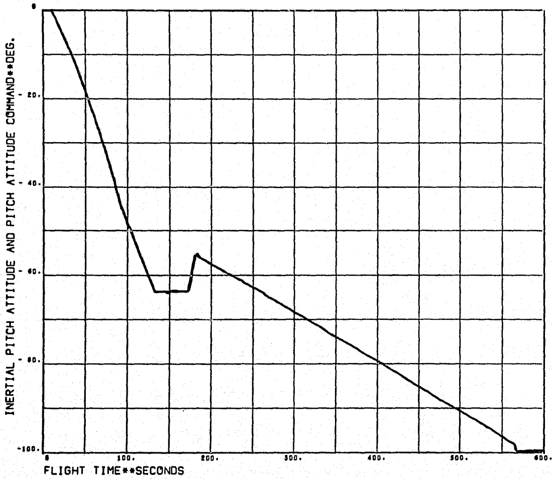
FIGURE 11C APOLLO/SOYUZ TEST PROJECT TYPICAL PLANAR CASE INERTIAL PITCH ATTITUDE AND PITCH ATTITUDE COMMAND HISTORIES
