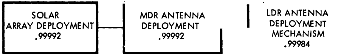
Figure 10-5. Reliability Logic Diagram of Structure and Mechanisms
