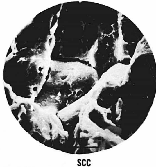
Fig. 94 SEM FRACTOGRAPHS OF TENSION AND SCC FRACTURE SURFACES T-L SPECIMENS OF 17-7PH RH1050 ALLOY
