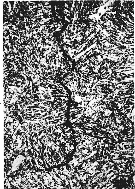
OXALIC ETCH OXALIC ETCH Fig. 78 PHOTOMICROGRAPHS OF CROSS SECTION ILLUSTRATING CRACK GROWTH AT MIDPLANE OF PH13-8 Mo H1050 ALLOY EXPOSED 141 DAYS TO SEACOAST ATMOSPHERE
