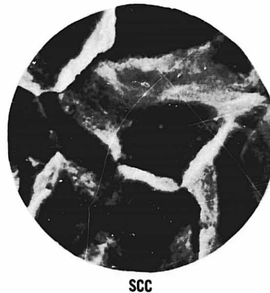
Fig. 95 SEM FRACTOGRAPHS OF TENSION AND SCC FRACTURE SURFACES IN S-L SPECIMENS OF PH13-8 Mo H1050 ALLOY
