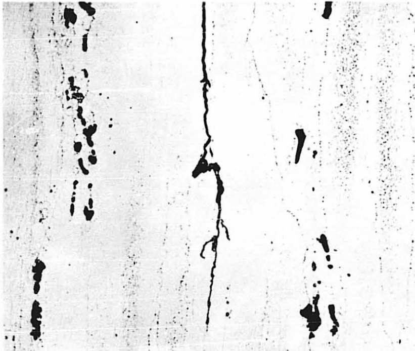
FIG. 19b HIGHER MAGNIFICATION (500X) OF THE REGION CIRCLED ABOVE SHOWING BOTH INTERGRANULAR AND TRANSGRANULAR TENDENCIES AT THE TIP OF THE CRACK (SEE FIG. 20).
