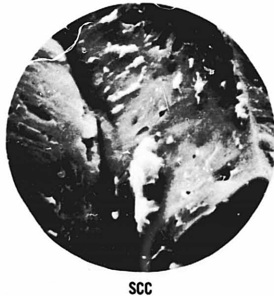
Fig. 96 SEM FRACTOGRAPHS OF TENSION AND SCC FRACTURE SURFACES IN T-L SPECIMENS OF 431 HT200 ALLOY
