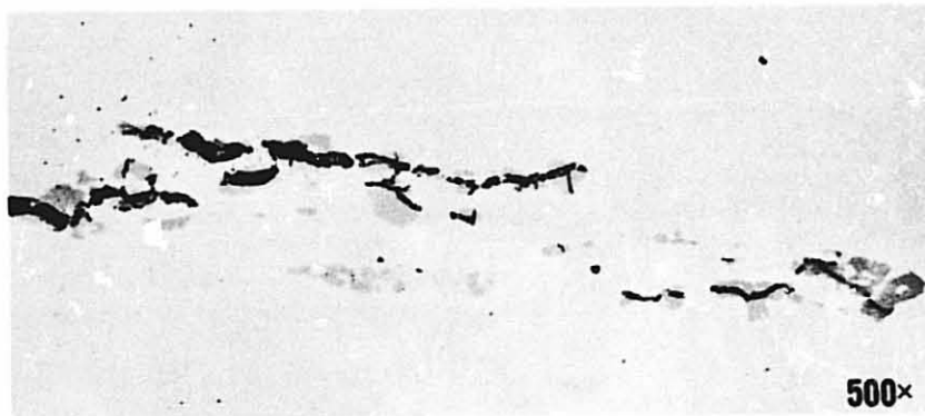
FIG. 46 S-L COMPACT TENSION SPECIMEN OF 2024-T851 BOLT LOADED TO POP-IN AND EXPOSED 1656 hr. TO SALT - DICHROMATE - ACETATE SOLUTION. SHOWS CRACKING OF ALLOY CONSTITUENTS AHEAD OF THE CRACK TIP.
