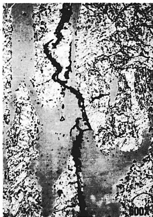
Fig. 77 PHOTOMICROGRAPHS OF CROSS SECTION ILLUSTRATING CRACK GROWTH AT MIDPLANE OF T-L SPECIMEN OF 17-7 PH RH1050 ALLOY EXPOSED 41 DAYS TO SEACOAST ATMOSPHERE
