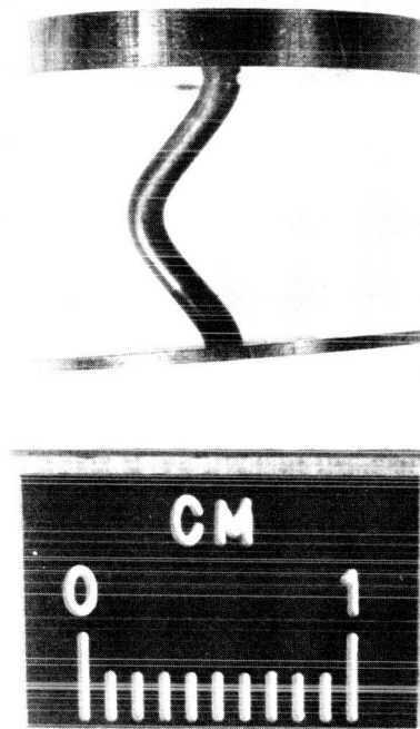
Figure 9. - T-111 vibration suppressor after failing during vibration test.
