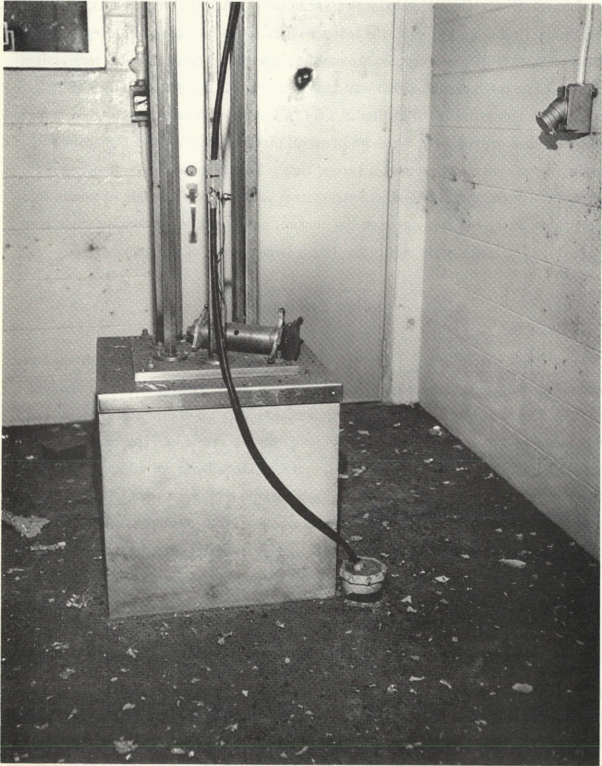
Figure 1. LOX Impact Test Cell after LOX/Asphalt Reaction.
