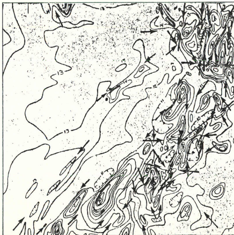
FIGURE 5B. U.S.G.S. aeromagnetic map at 1:250,000 scale of the Canaan, Connecticut test site. Arrows point to linear magnetic anomalies and anomaly separations which correlate with fractures mapped from ERTS-1 and SLAR imagery.
