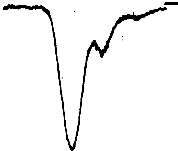
Figure 2. - Waveform (1 ns per division) as passed through complete system, with receiving horn facing the transmitting horn.
