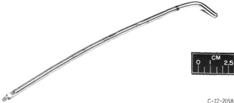
Figure 12. - Failed spindle of drive turbine.
